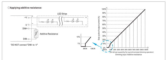
Note : 1. Min. duty cycle of output current is about 1%, and the dimming input is about 6KΩ or 0.6VDC, or 10V PWM signal with 6% duty cycle.
